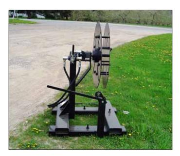
This unit was designed to rewind wire from trellis and grape plantings where it is no longer needed. The wire winder also winds the wire into standard coils so it can be reused in new plantings.
